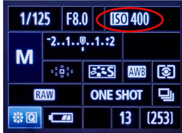
Example of how the ISO setting might appear on an LCD display
